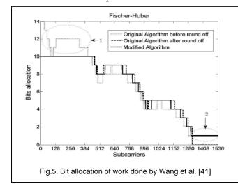
The outcome of the study is shown in Fig.5 and Fig.6 for bit allocation performance and for BER performance respectively. The comparative analysis is done with original Fischer and Huber algorithm with the modified one.
